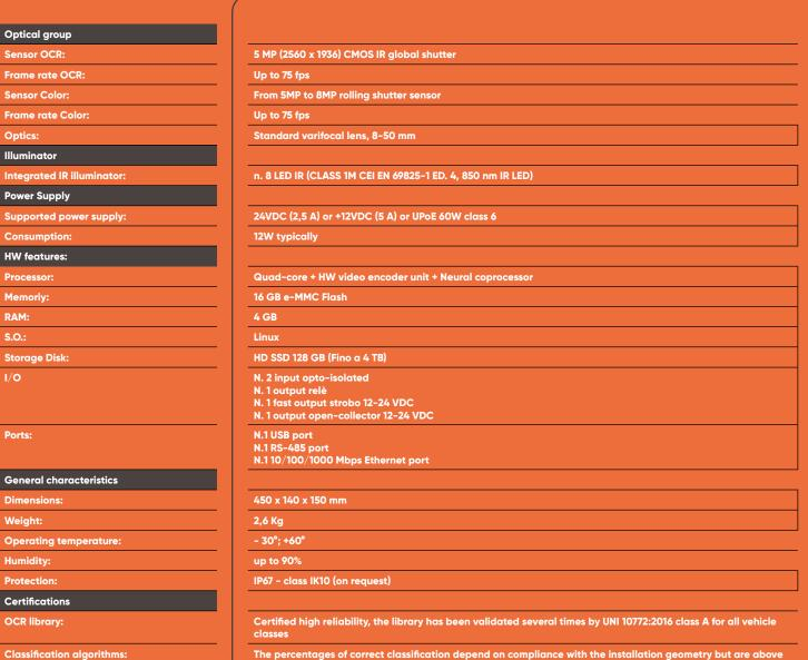
The percentages of correct classification depend on compliance with the installation geometry but are above 90% regardless of the external environmental conditions
